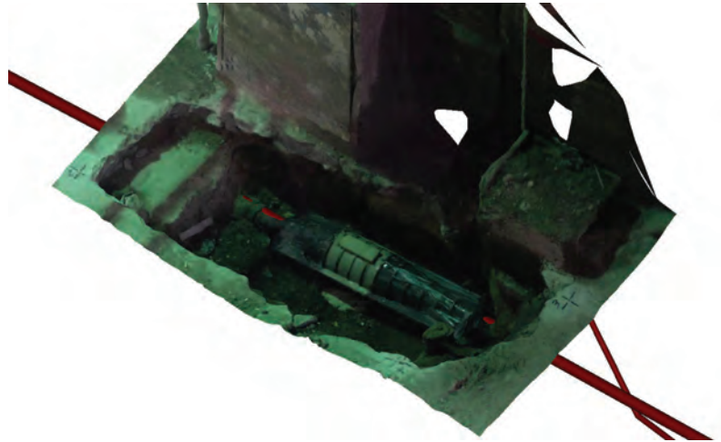
Figure 1: 3D view of a photogrammetric model of an excavation (Follow the link to: https://www.youtube.com/watch?v=wtrpxqEAt9k )
