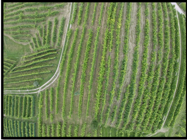
FIGURE 11 - IMAGE OF THE VINEYARD COLLECTED IN THE RGB BANDS. IS POSSIBLE TO DISTINGUISH THE DISTORTION CREATED BY THE FISH-EYE LENS.
