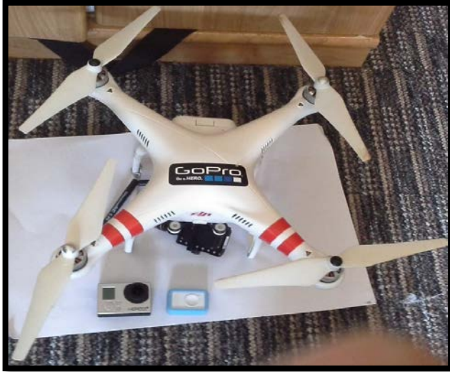
FIGURE 5 - DJI PHANTOM 2 MOUNTING THE GIMBAL. BELOW IS POSSIBLE TO SEE THE GOPRO CAMERA (LEFT) AND THE GEOTAGGER (RIGHT).
