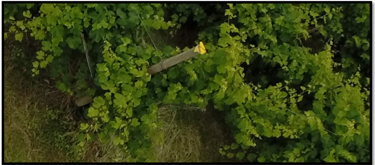
FIGURE 9 - ONE OF THE YELLOW PLASTIC WRAPS USED TO VISUALISE THE GROUND CONTROL POINTS ON THE IMAGES
